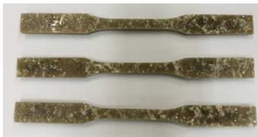
Fig. 3. View of specimens used in research: a) composite without recycle, b) composite with 10% of recycle.
