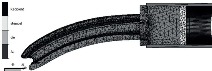
Fig. 2. Profile bending in symmetry plane of die for assumed process parameters
