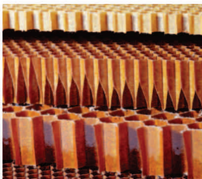
Fig. 2. Composites reinforced with amide fibers with a macromolecular structure
