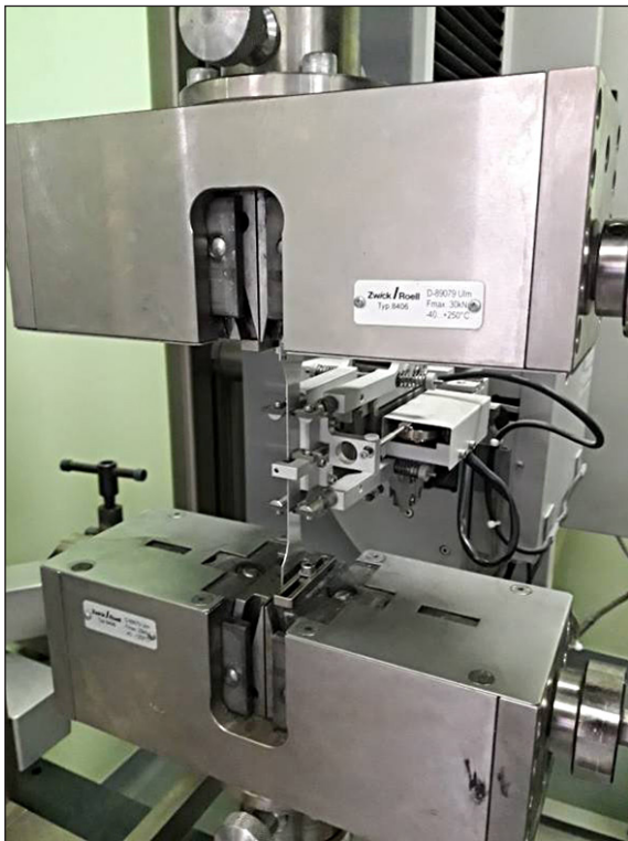
Fig. 4. An example of a sample during the uniaxial tensile test
