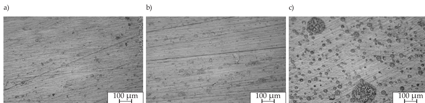
Fig. 4. Optical micrograph of compositions modified with ETBN (magnification 320x): a) 2 phr premix, b) 6 phr premix, c) 10 phr premix
