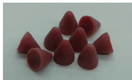
Fig. 2. Polyester media, cone with dimensions: diameter 14 mm, height 14 mm
