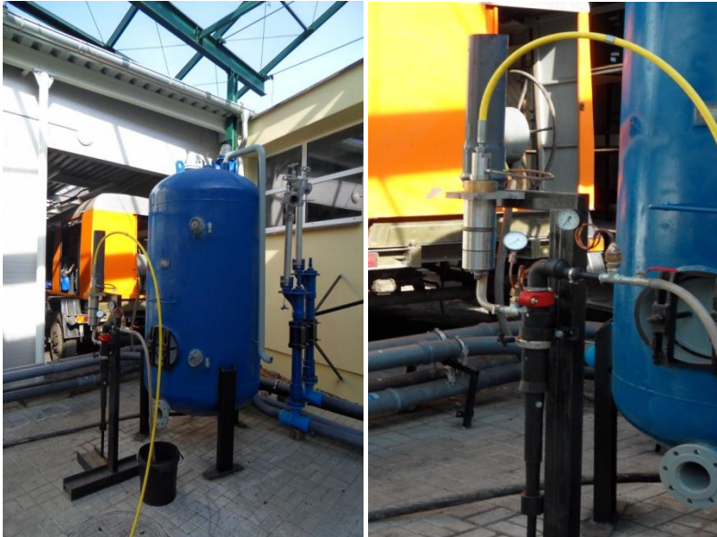
Fig. 1. General and detailed view of hydrojetting comminution apparatus prototype
