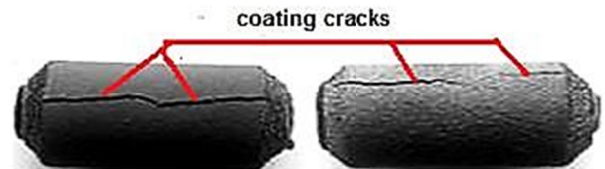
Fig. 4. View on the coatings sprayed on steel rollers by hybrid method with injector type B40 consisting of two micro-steam diameter of 40 μm
