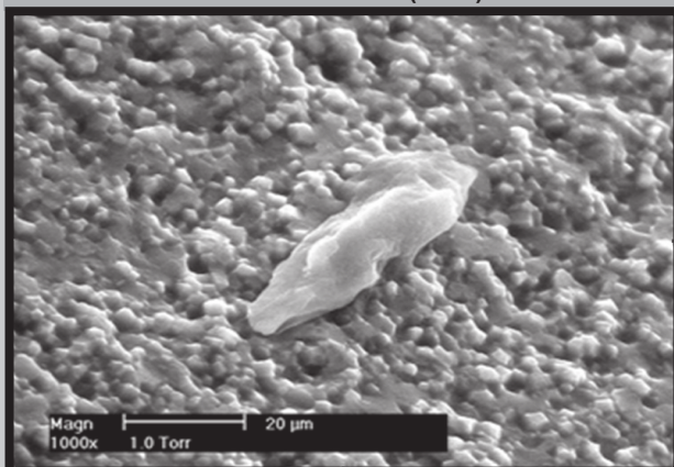
FIG.3. The view of the surface with biofilm (1000x)
