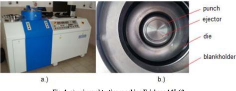
Fig. 1. a) universal testing machine Erichsen 145-60, b) tool set for deep drawing cup test [source: own study]
