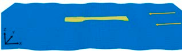
Figure 10. Irregular wave and coordinate system of seakeeping analyses
