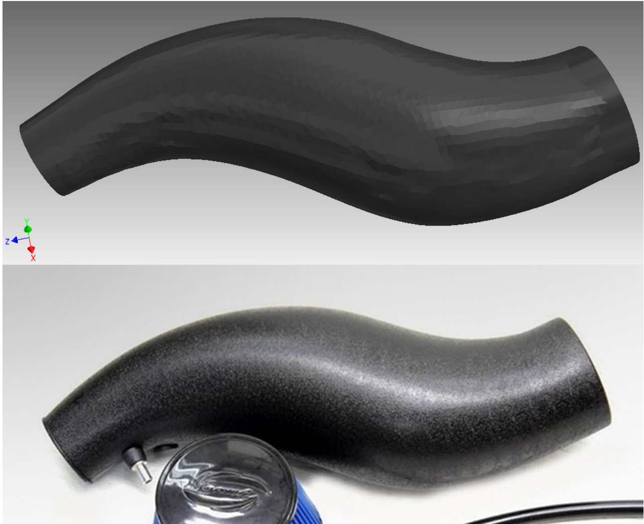
Fig. 3. Real intake unit geometry (lower) [8] versus obtained geometry (upper)
