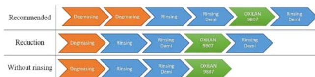
Figure 5. The stages of the process of washing and degreasing OXILAN 9807 depending on the type of the process
