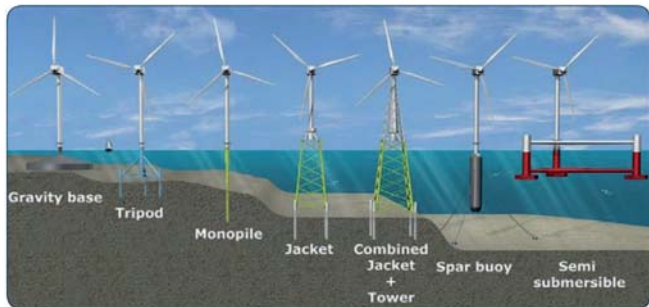
Fig. 1. Various solutions of anchoring the offshore wind power electric plants, depending on water depth [3]
