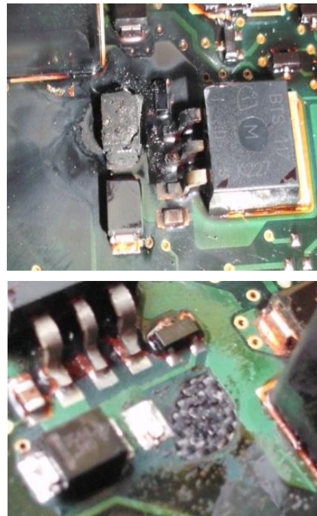
Fig. 6. On the left damaged part on board controller, to the right view of plate after cleaning
