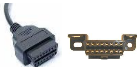
Fig. 4. Standardized 16-pin connector on boarding diagnostic EOBD [11, 23-26]
