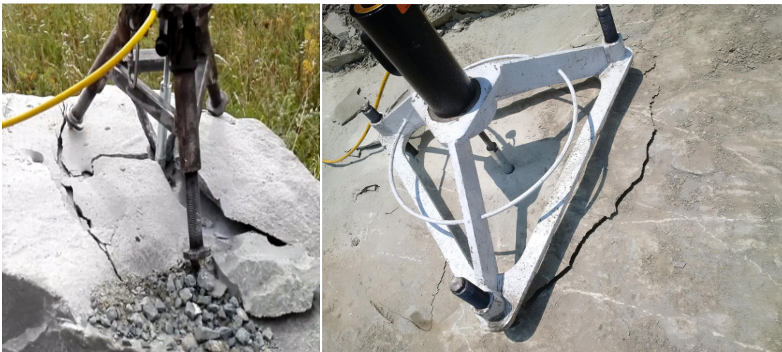
Figure 13: Pull-out test performed on actual rock (Jonak et al., 2019).
