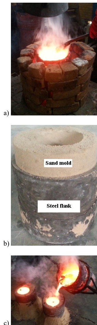
Fig. 1. Equipment used in the research, which are available in Payvaran Parsian Company, a) Induction Furnace, b) Sand Mold, c) Pouring
