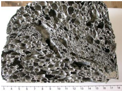
Fig. 2. Shapes of aluminum foam pores
