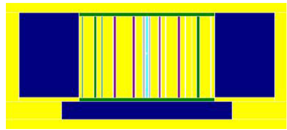
Fig. 2. Vertical cross section of MNSR reactor using the MCNP4C code.
