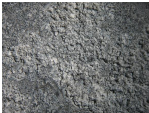
Fig. 7. Surface topography of alloy 2 sample (after 6 h of being immersed in 5% NaCl solution, 7x)
