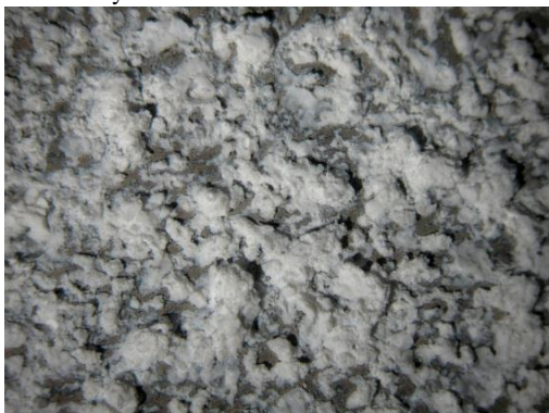
Fig. 6. Surface topography of alloy 1 sample (after 6 h of being immersed in 5% NaCl solution, 7x)
