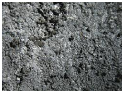
Fig. 8. Surface topography of alloy 3 sample (after 6 h of being immersed in 5% NaCl solution, 7x)
