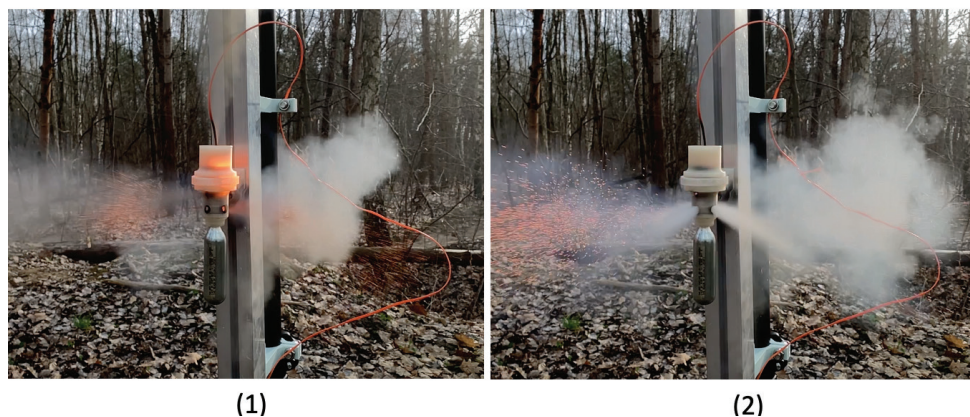
Fig. 9. Operation test of the first designed parachute ejection mechanism: (1) – moment of ignition of the pyrotechnic igniter charge; (2) – moment of puncture of the CO 2 cartridge membrane and release of compressed gas.
