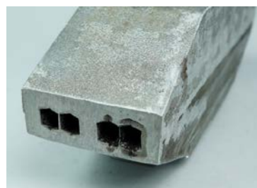
Fig. 10. Detail of the resulting heat exchanger casting
