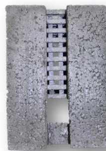
Fig. 13. Cleaned casting, material AlSi10MgMn CSN 424331, bottom view [22]
