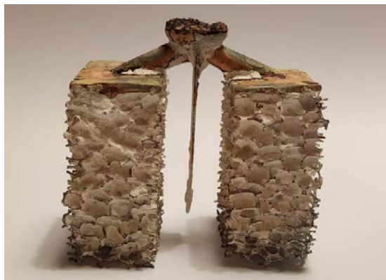
Fig. 4. Casting after gypsum mould breaking
