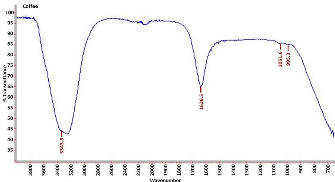
**Figure 3.** FTIR spectrum of used coffee grounds extract
