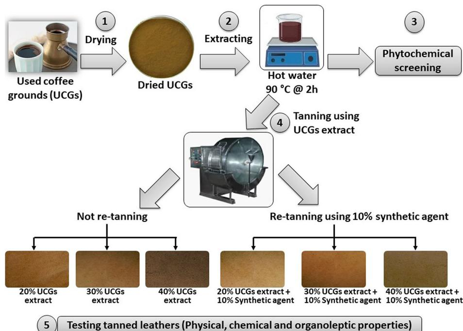
**Figure 1.** Schematic diagram for working steps
