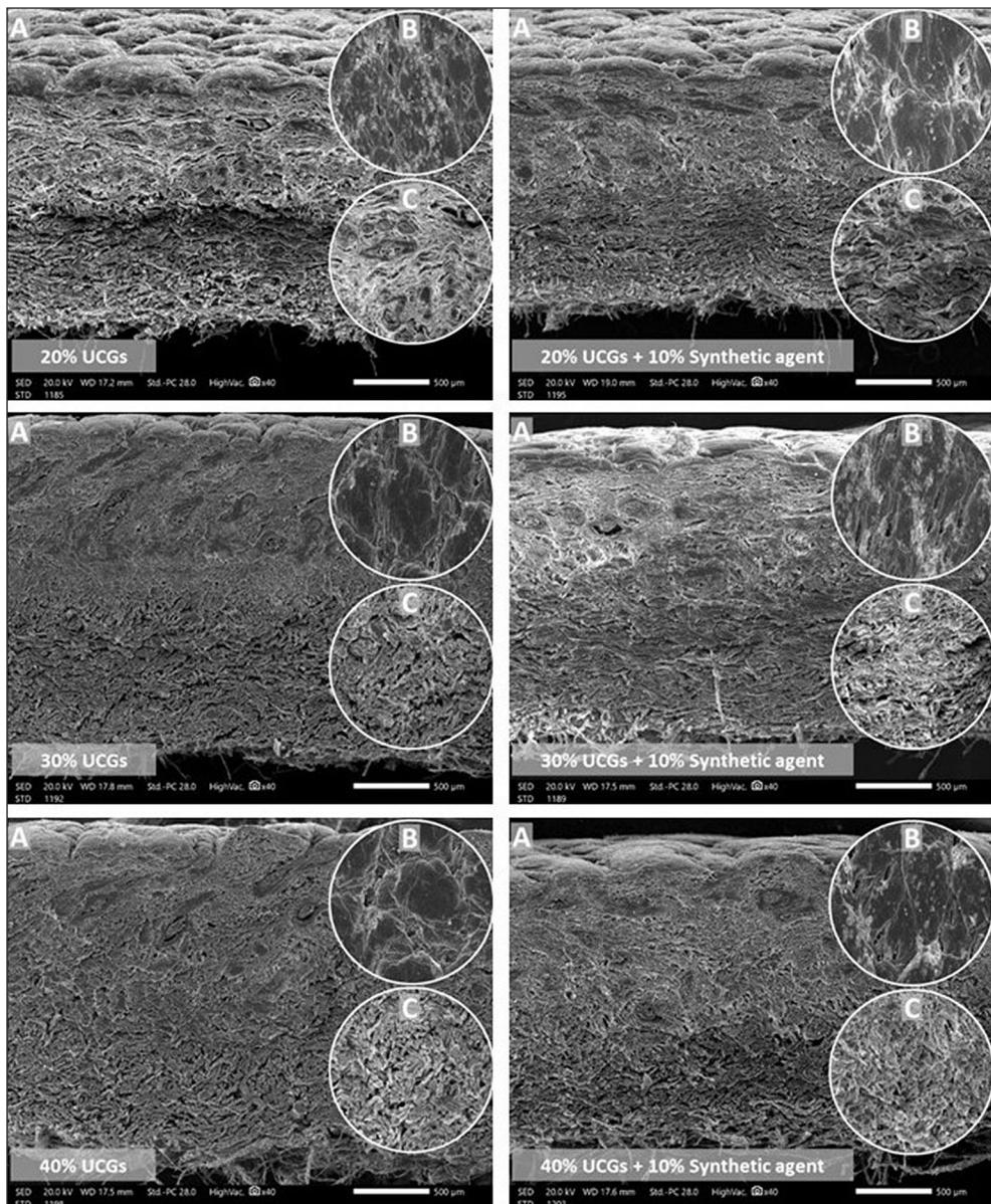
**Figure 4.** Scanning electron micrographs for all tanned leathers groups with used coffee grounds (UCGs); (A) cross section depicted at x40, (B) grain surface depicted at 100x, and (C) collagen bundles depicted at 150x
