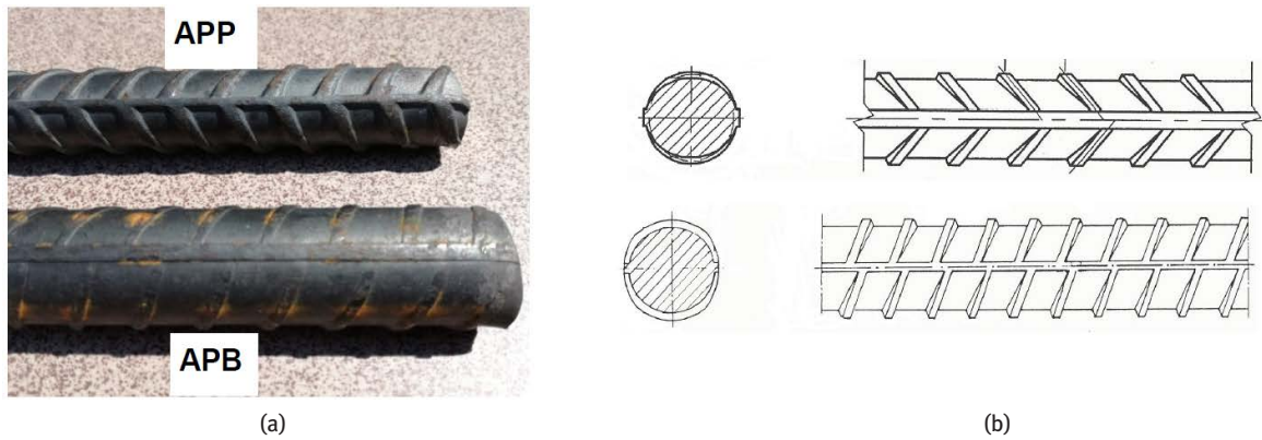
Figure 8: APP and APB-type bolt rods (a) and cross section diagrams (b).
