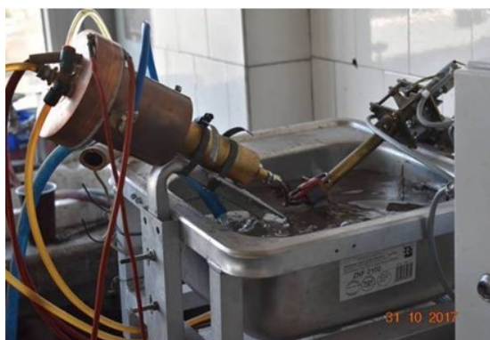
Fig. 1. A device for simulating heat shock
