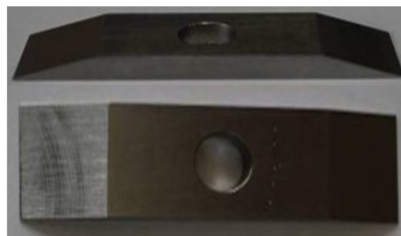
Fig. 2. Sample for evaluation of the resistance to thermal shocks
