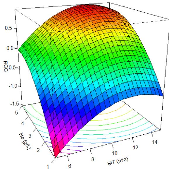
**Figure 7.** Estimated response surface for chromium removal in CE
