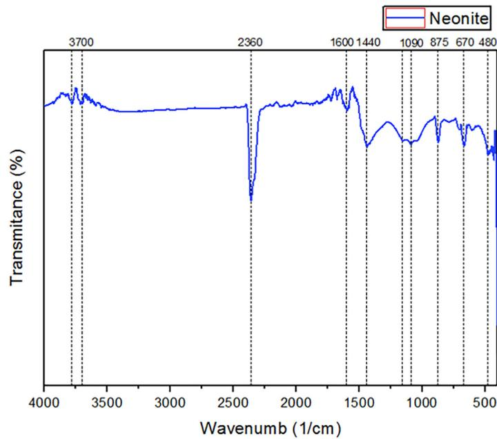
**Figure 1.** FTIR characterization of Neonite
