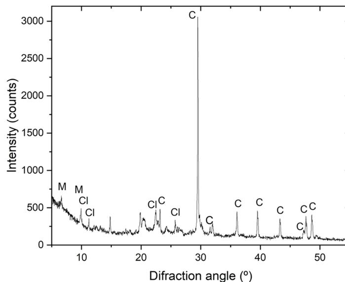
**Figure 2.** XRD characterization of Neonite
