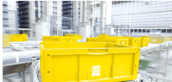
Fig. 2. Roller conveyor sorting system [Source: ssi-schaefer.com]
