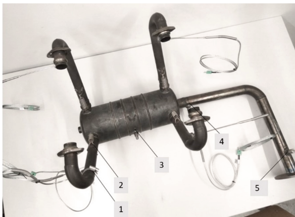
Fig. 3. Exhaust system of ROTAX 912 ULS engine
