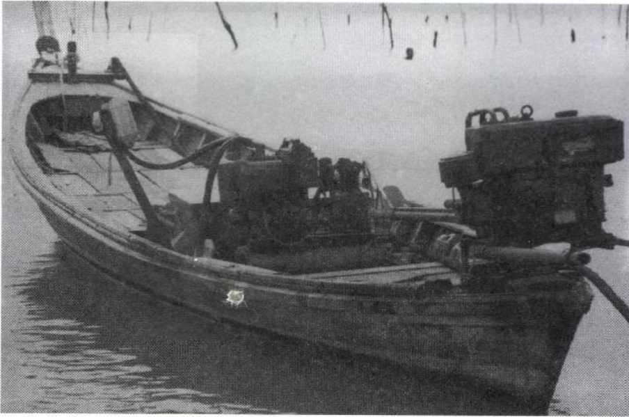
Figure 1. The traditional dive boat with the compressor located in the middle of the boat.
