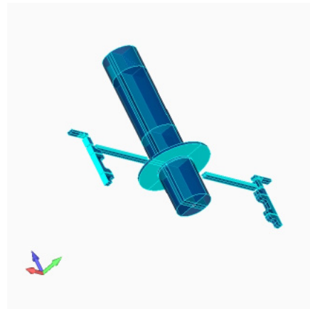
Fig. 4. Fragment of MOD-AE model, including shaft, caps, and transverse ribs
