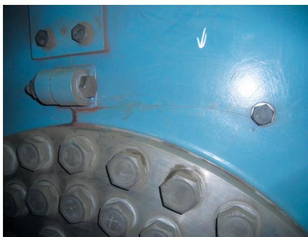
Fig. 1. Side disc cracks above the hub
