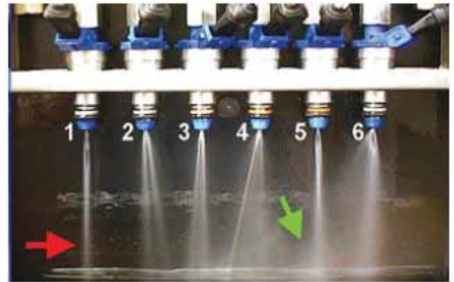
Fig. 7. Pattern of possible disturbances in injectors' operation – full set from the same engine [www.intercars.com.pl]
