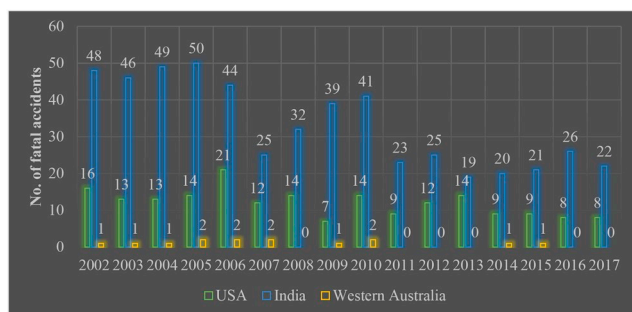
Fig. 1. Comparison of the number of fatal accidents in Indian underground coal mines with the USA and Western Australia.
