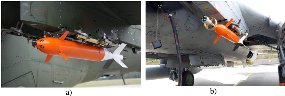
Fig. 2. Prototypes of guided bombs: a) inertial seeker; b) external wind stabilised seeker
