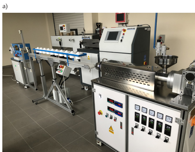
Fig. 1. Designed as part of the work, an original filament production line
