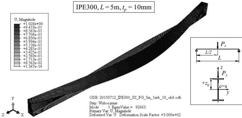
Fig. 3. Exemplary beam modelled using the Abaqus software
