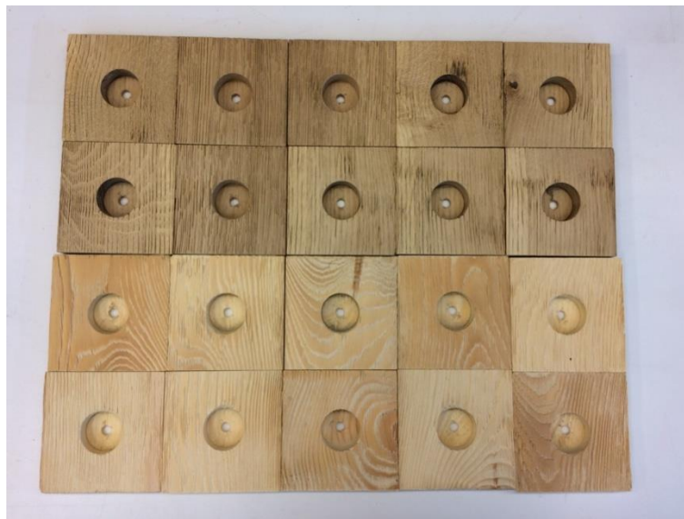
Figure 5. Samples after brushing: oak wood (row 1 and 2) and pine wood (row 3 and 4)
