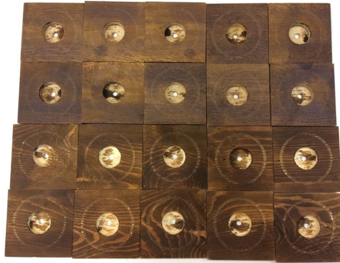
Figure 6. Samples dyed with potassium permanganate: oak wood (row 1 and 2) and pine wood (row 3 and 4)
