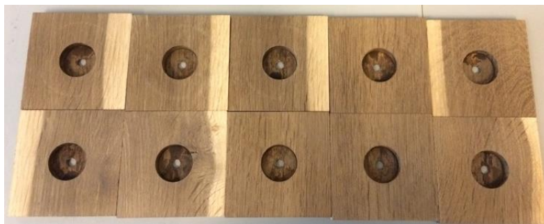
Figure 7. Oak wood samples dyed with ammonia fumes
