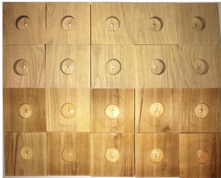
Figure 1. Zero samples of oak wood (row 1 and 2) and pine wood (row 3 and 4)
