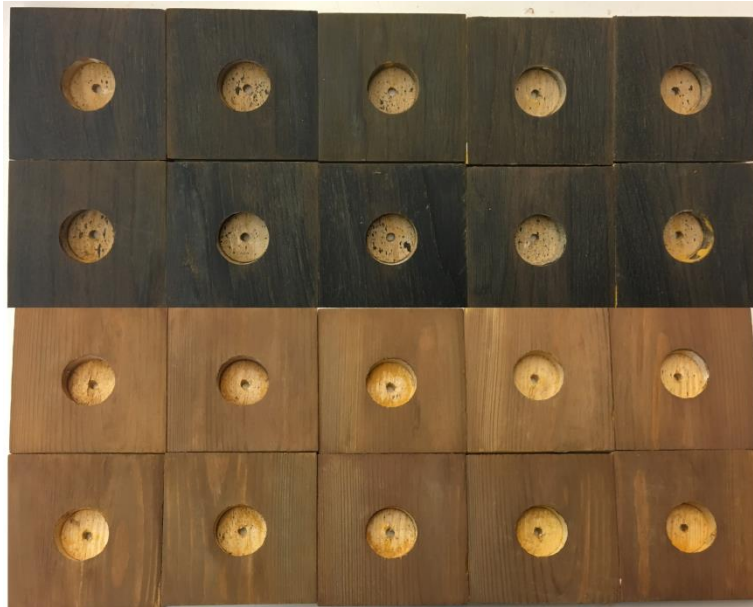
Figure 4. Greyed samples: oak wood (row 1 and 2) and pine wood (row 3 and 4)
