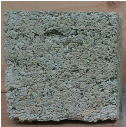
Fig.1. The sample of hemp-lime composite [authors' archive]
