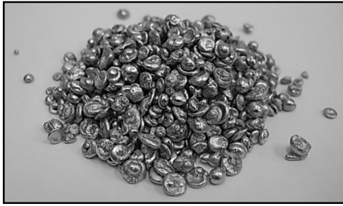
Fig. 3. Granules of CuAl10Fe5Ni5 bronze cast on INDUTHERM-VC 500 D Vacuum Pressure Casting Machine according to the plan of the experiment E_3(1180.116)
