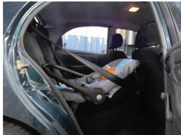
Fig. 5. Safety seat with the BABY dummy, installed on the rear seat
