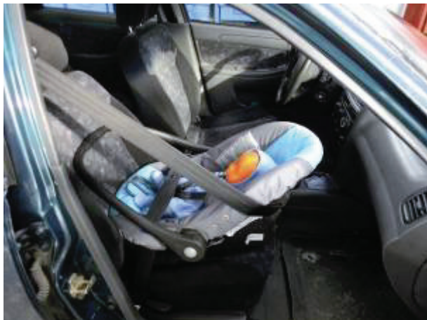
Fig. 4. Safety seat with the BABY dummy, installed on the front seat
