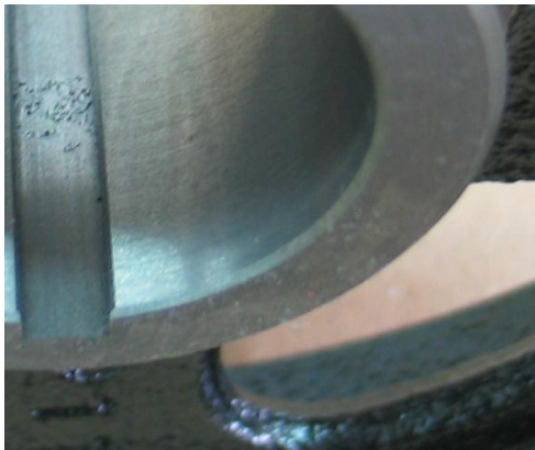
Fig. 4. Porosity of casting
