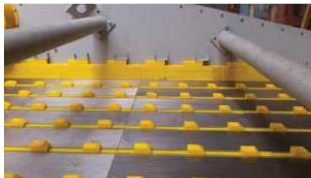
Fig. 14. Sieve deck, slotted, welded, built-in PRO-CLIN system
