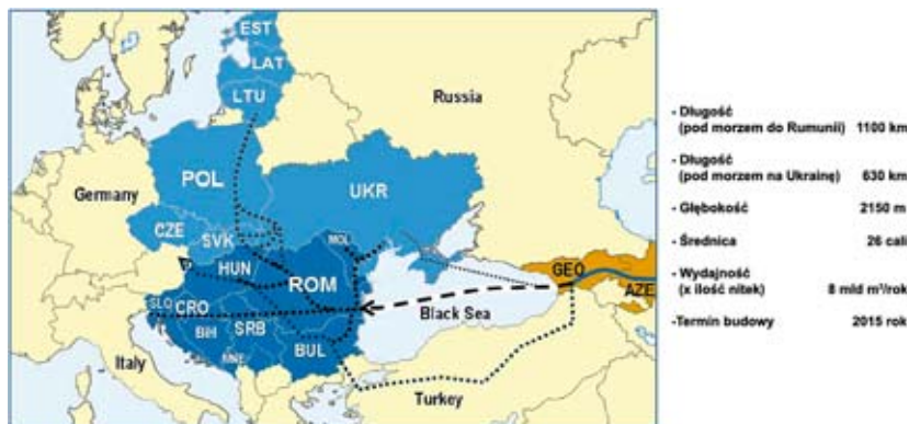
Rys. 6. Projekt i trasa gazociągu White Stream, wg. 2009 GUEU – White Stream Pipeline Company Limited, the White Stream Corporation
