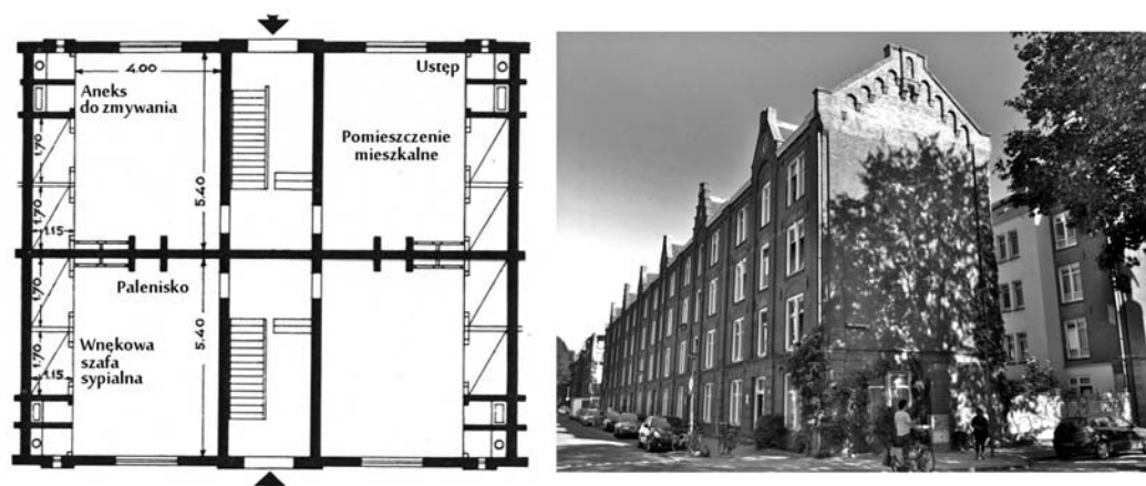
Fig. 12. Amsterdam. „Back to back” building. Projection of the ground floor – on the left (Marnixstraat) and building D – on the right (Blankenstraat 2-12, B. de Greef, 1878–1881). Source: [10, p. 29 (on the left), 2 (on the right)]
