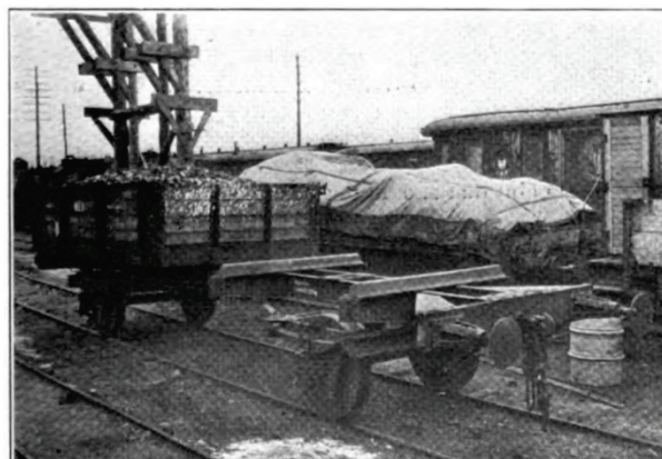
Container Car with One Body Removed Showing Details of Underframe
