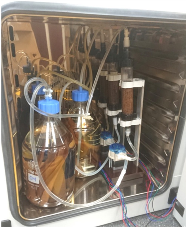
Fig. 6. Three measuring systems placed in a heat chamber used for drying cellulose materials impregnated with mineral oil, natural ester, and synthetic ester
