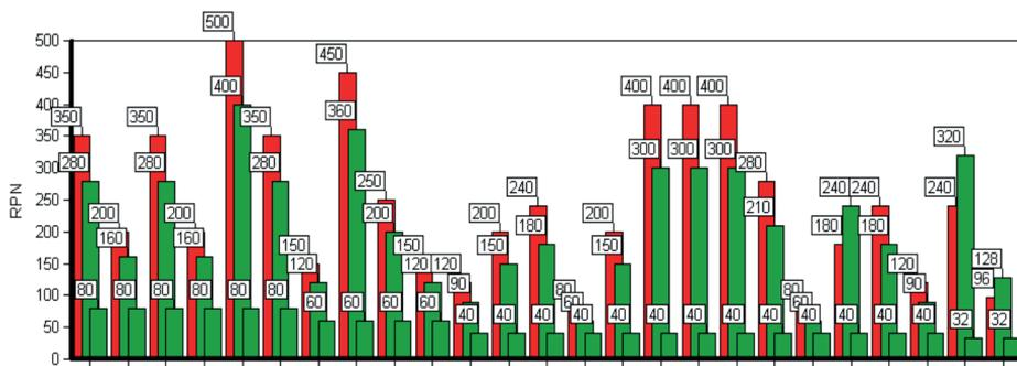
Fig. 4. RPN values for existing and proposed maintenance system
