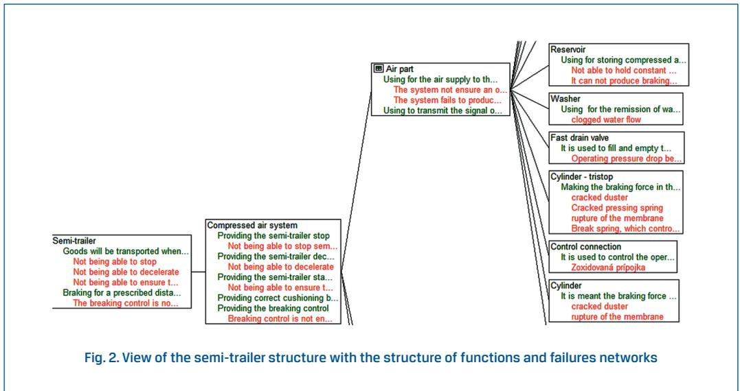
Fig. 2. View of the semi-trailer structure with the structure of functions and failures networks
