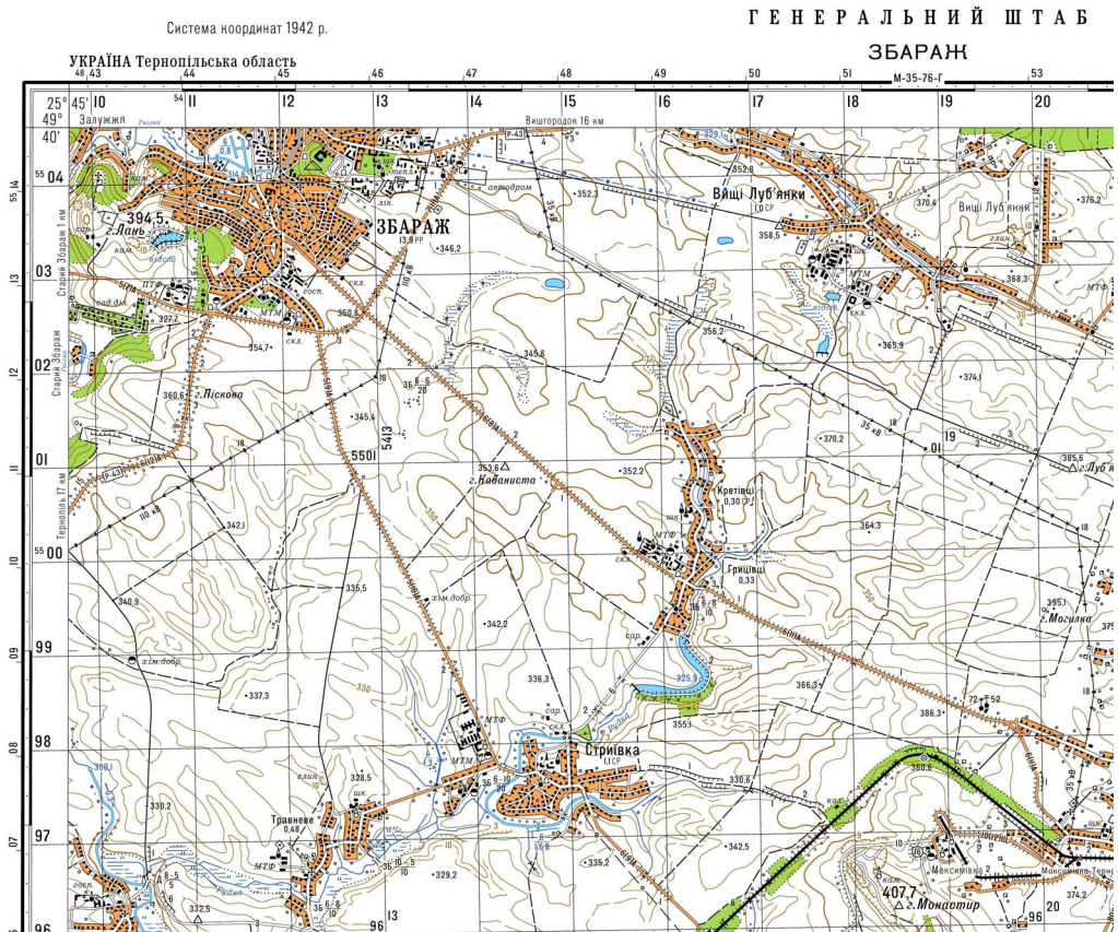
Fig. 5. A part of the traditional 1:50,000 scale topographic map (made according to the instructions for topographic maps)
