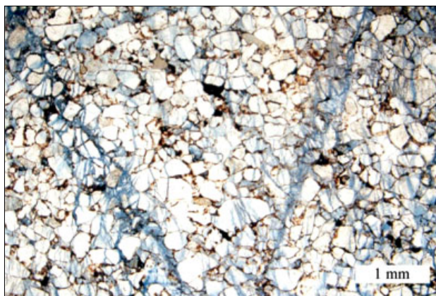
Pic. 4. Failure zones of sample ( \sigma_3 = 250 MPa; \varepsilon_1 = 10\% ), enl. \times 25
