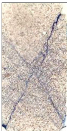
Pic. 3. Zone of destruction of the sample, microscopic section ( \sigma_3 = 250 MPa; \varepsilon_1 = 10\% )
