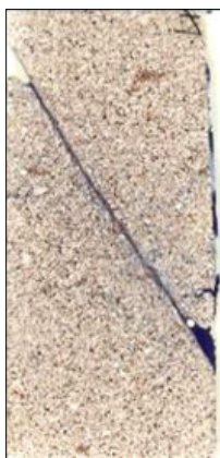
Pic. 1. Sample's cracking, microscopic section ( \sigma_3 = 125 MPa; \varepsilon_1 = 20\% )
