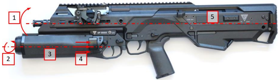
Photo 4. Forces and moments acting on the carbine-grenade launcher configuration when firing a grenade launcher round (courtesy: FB Radom): (1) direction of bending moment; (2) direction of torsional moment; (3) grenade launcher centreline; (4) direction of recoil forces; (5) rifle centreline
