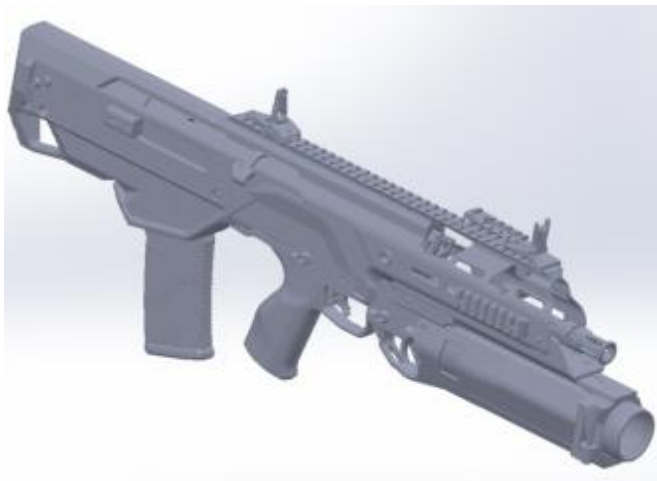
Fig. 1. CAD model of the rifle and the under-barrel grenade launcher before optimisation
