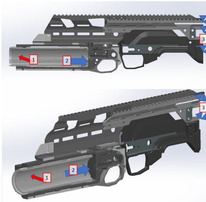
Fig. 4. The method of constraint and input loading applied in the calculation model: (1) input by forces acting to the barrel grooves; (2) input by the pressure behind the projectile in the barrel; (3) constraint of the calculation model in directions x, y, and z
