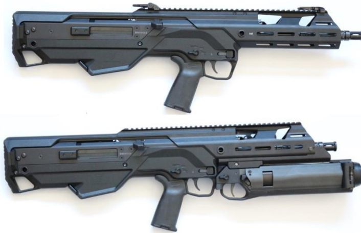
Photo 2. MSBS-5.56B bullpup rifle prototype without a grenade launcher (top) and with the 40 mm calibre under-barrel grenade launcher (bottom) (FB Radom)
