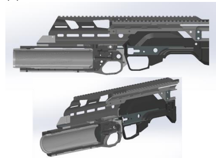
Fig. 2. Numerical calculation-optimised CAD model of the rifle with its under-barrel grenade launcher: (a) post-simplification model overview; (b) removed portion of the rifle; (c) cross-sectional view of the simplified model
