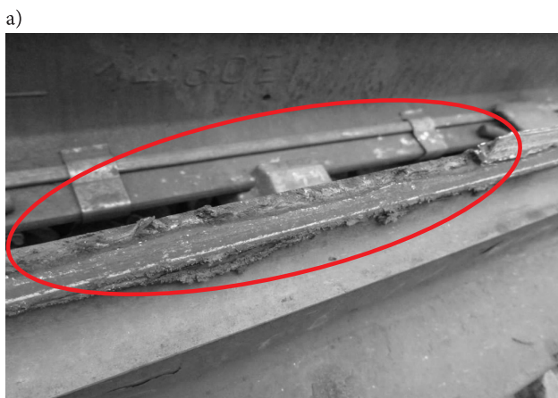
Fig. 3. Damage to switch rails in the form of spallings of material a) and b) [photo. M. Czarnecki]
