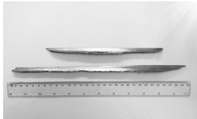
Fig. 5. Switch rail spall material [photo. M. Czarnecki]
