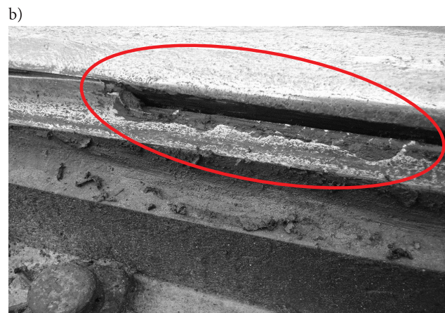
Fig. 3. Damage to switch rails in the form of spallings of material a) and b) [photo. M. Czarnecki]
